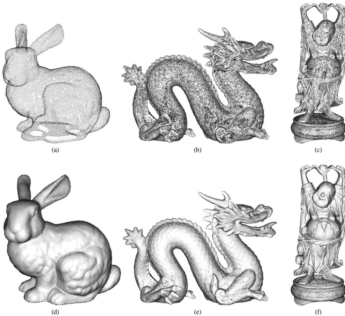
Fig. 11. Three large complex point sets from the Stanford 3D scanning repository. (a) The Bunny model. (b) The Dragon model. (c) The Buddha model. (d)–(f) are the rendering models corresponding to (a)–(c).
